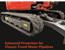
The AX-18 features travel motor hoses enclosed within the track frame, a design choice that significantly cuts repair costs and boosts durability, showcasing our commitment to thoughtful engineering and long-term value.
